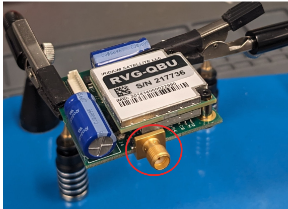
Figure 7.11: RockBLOCK module before removing the SMA connector (circled).
