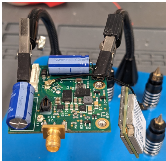
Figure 7.12: RockBLOCK module after removing the Iridium 9603 modem.
